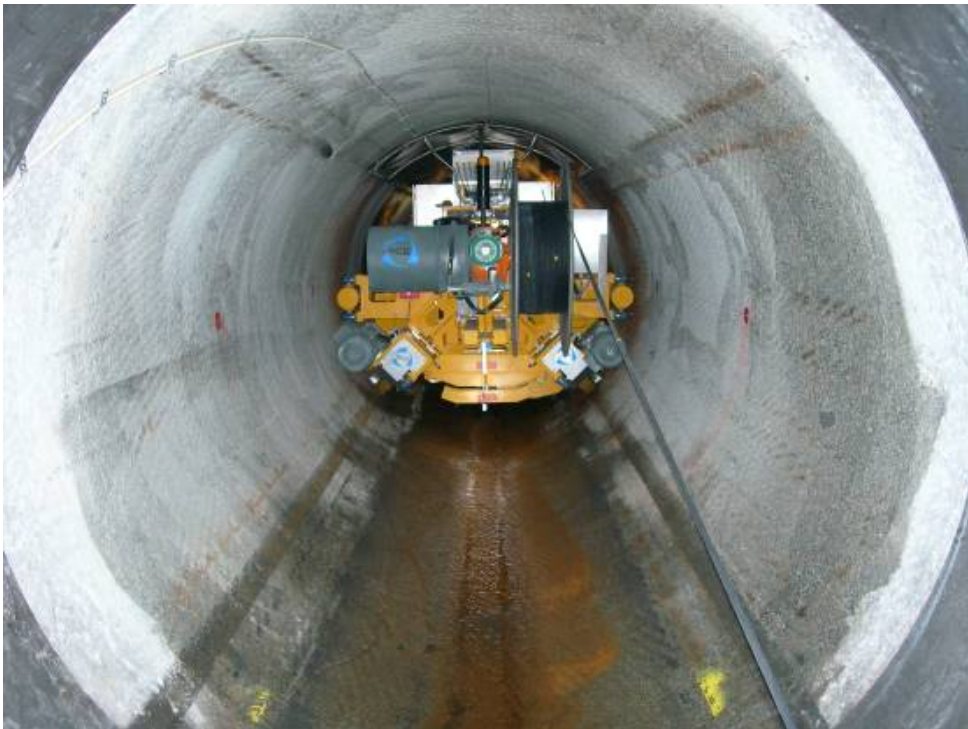
Figure 4-1. The KBS-3H deposition machine inside the horizontal deposition hole.
