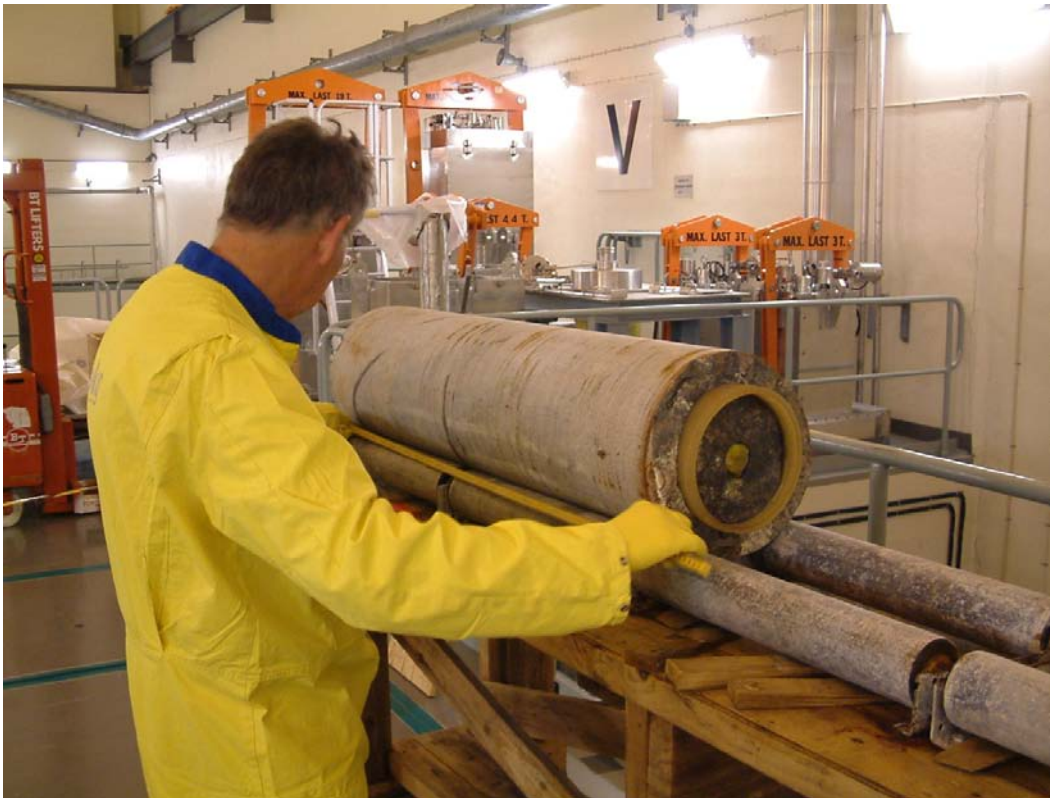
Figure 3-2. Geological mapping of the 278 mm diameter core from LTDE-SD, including the 177 mm diameter core stub and rock surrounding the small diameter extension borehole.
