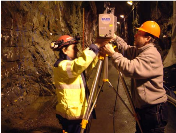
TASQ-tunnel, mounting of the Faro laser scanner used by ATS (photo Björn Magnor)
