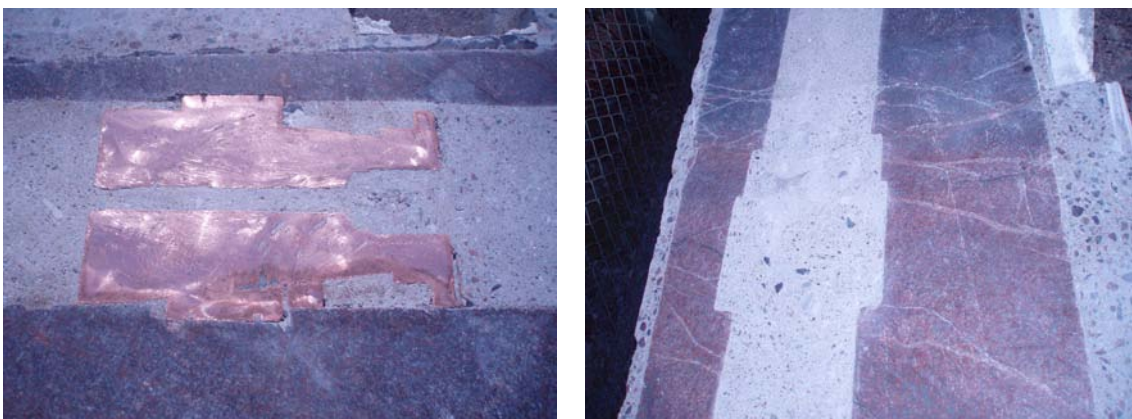
Figure 4-5. Over cored copper plug (left) and quartz/cement plug (right).
